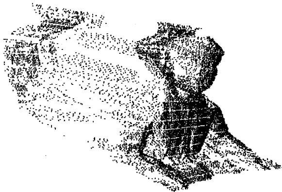
Fig. 3. Example of 3D reconstruction of a teleconferencing scene from three calibrated views. From top to bottom: one of the original views; progressive refinement of the reconstructed surface, final cloud of points after outlier thresholding.
