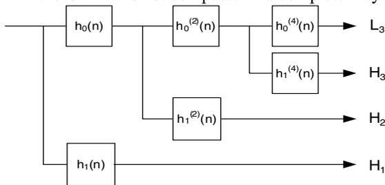
**Figure 5 - Overcomplete DWT (ODWT) computed through the algorithm à trous.  $h^{(k)}(n)$  is the dilated version of  $h(n)$  obtained inserting  $k-1$  zeros between two consecutive samples.**
