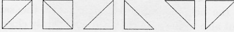
Figure 13: Six possible configurations for the creation of triangles from four neighboring points.
